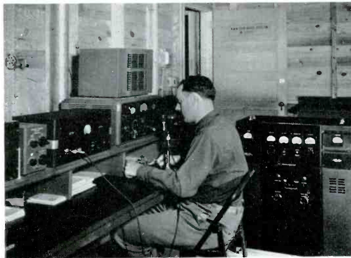
Uncle Sam's Own Ham Station — First Lieut. P. W. Simms, Officer in Charge, at the mike of one of the two completely equipped operating positions of W20EC, Army owned ham station. Hallcrafters equipment, left to right is: HT-7 Frequency Standard, HT-5 speech amplifier, SX-28 communications receiver and HT-4 transmitter (in console cabinet at right of operator).
